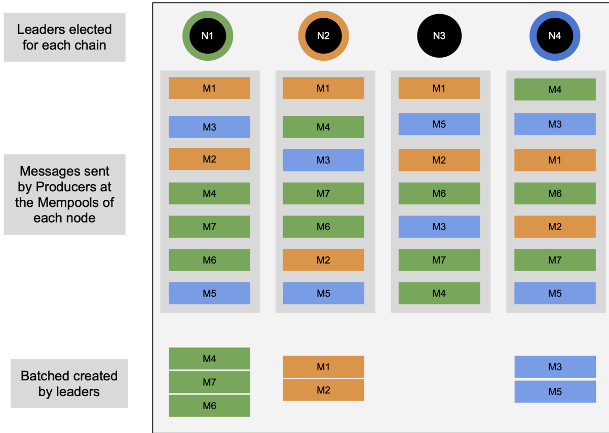
Fig. 1. Mempool data structure for four nodes are illustrated alongside chain based leader designations for each of the nodes. Messages of the same color belong to the same chain. N1 , N2 , N3 are leaders for the chain 1 (green), chain 2 (orange), chain 3 (blue) respectively
